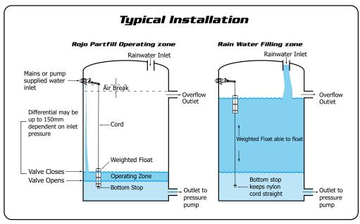
Note: Keep overflow, rain water inlet and outlet to pressure pump as far away from the float valve as possible.
